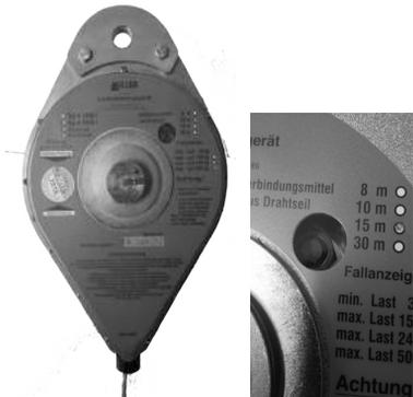
Fig 2: fall indicator original at the device
